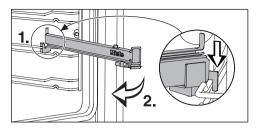
Hook the FlexiClip runner onto the front of the top rail of a side runner (1.) and then hold it at an angle in towards the middle of the oven compartment (2.).
